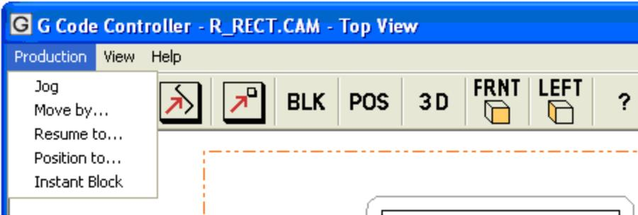
This illustration shows how the **Production** menu may appear after the **Run** (or **Dry Run**) **Tool Path** dialog has been opened. Manual motion dialogs are accessible, including **Resume to**, which provides assistance positioning the **Stages** to a resuming position along the tool path. Dialogs that affect initializing the **Machine Home** position: **Set Home** and **Limit Switch Seek**, are absent in this context.
